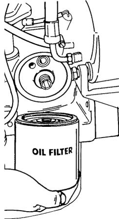
2. Coat sealing ring on new filter with engine oil and install the filter.
