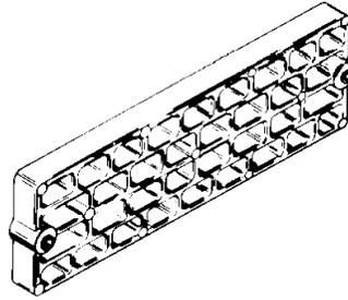
**Trim Cylinder Anodes** - are mounted on each trim cylinder.
