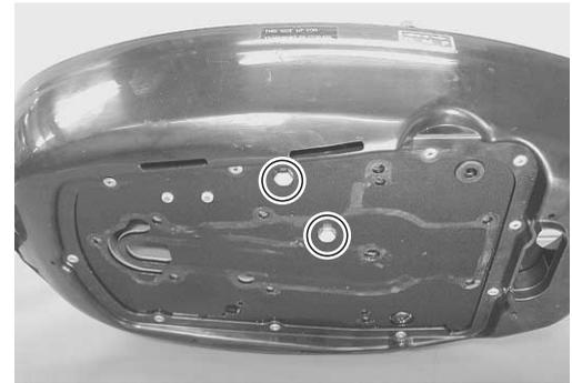
17. Remove the cushion rubbers and the oil filler cap.
