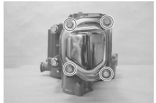
2. Loosen the four cylinder head bolts in the order indicated and remove the bolts.
