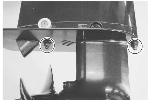
5. Remove the cotter pin and the propeller nut, then detach the propeller.
