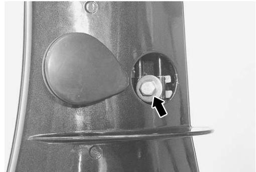
3. Remove the two nuts and washers. (for the transom "L" model)
