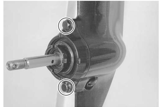
8. Remove the propeller shaft bearing housing.
