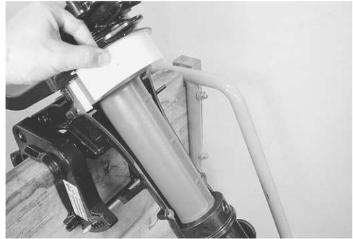
11. Remove the two bolts, the steering bracket and the bracket cover.
