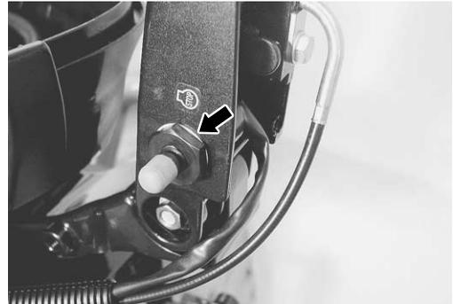
4. Remove the pivot nut and the washer.
