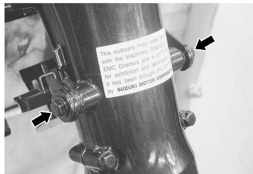
8. Remove the reverse lock arm and the springs.
