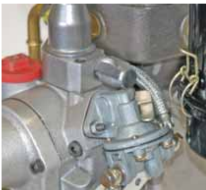
Fig. 30: Example: automatic decompression with lever
