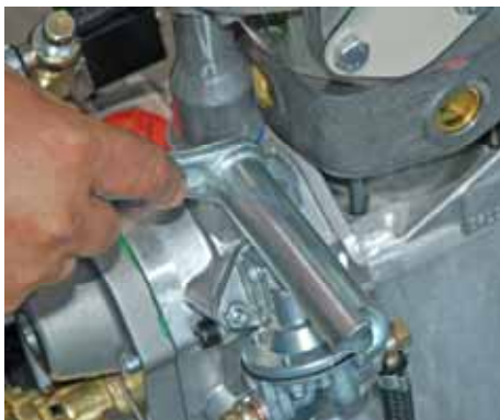
Fig. 32: Example: Adjusting the automatic decompression on the starting handle with the adjusting spanner
