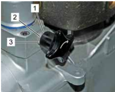
Fig. 29: Example: automatic decompression with star knob
