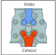
The intake and exhaust passages are short and straight for maximum airflow at all RPM's providing for high power output and no smoke. The short intake ports don't add heat to the incoming air charge, improving performance. The short exhaust ports allow the engine to maintain heat energy. Maximum
