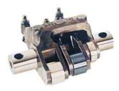
The overhead cam is able to operate each unit fuel injector directly, via a rigid rocker arm. Other engines, with the camshaft located in the block, use pushrods. This overhead system provides excellent stiffness for high injection pressures. The overhead cam in the Series 60 is capable of injection pressures over 30,000 PSI. High injection pressure means rapid start up, high power output, low smoke and emissions, instant throttle response and excellent fuel economy.
