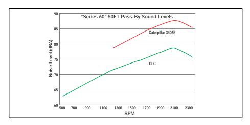
Another way to equate the level of noise: According to a recent advertisement by Caterpillar\*\*, they stated the interior noise level of a Cadillac STS is 72 dBA. You can see how well Series 60 engines measure up.
